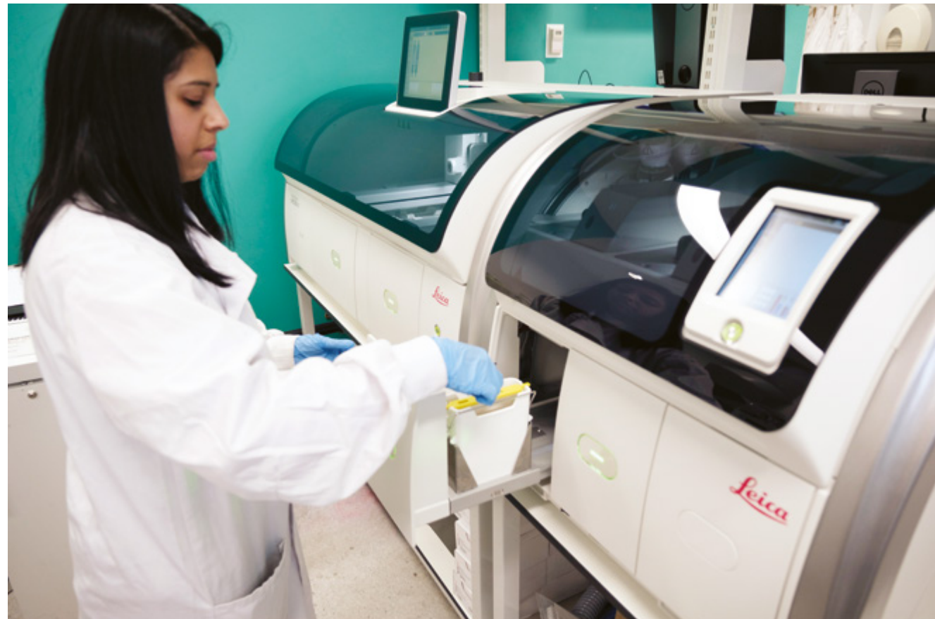
Aanzi Albert, Biomedical Scientist with a hematoxylin and eosin (H&E) stainer, which processes pathology slides.
